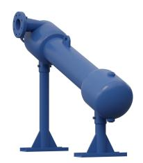
**Clemons Sand Separators** are ideal for removal of suspended solids and inorganic materials with a specific gravity of 2 or greater. This highly effective system will provide consistent, simple removal of inorganic material down to 75 microns. Easily installed, these carbon steel units are rated to 150 psi with threaded or flanged inlet/outlet connections. Smaller models are designed for vertical installation while larger models are angled and floor or ground mounted.
